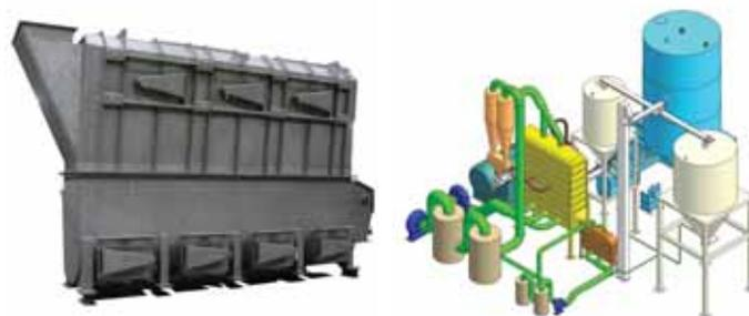
Schwing Bioset's fluid bed dryer offers a thermally efficient means of producing dust-free Class 'A' biosolids. Automated to allow unattended operation, the Fluid Bed dryer operates under completely inert conditions and, unlike other technologies, it does not require any recycle of already dried biosolids.
